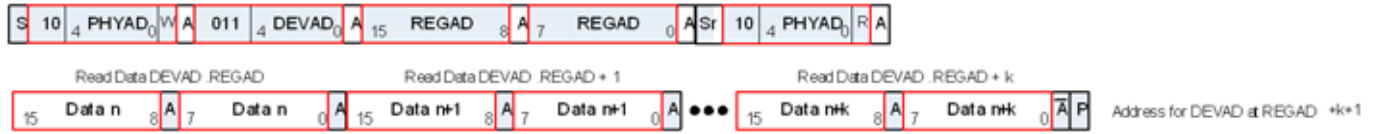
Figure 18: Read, Full Header, Post-Increment
