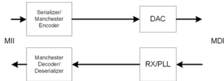
Figure 34: 10BASE-Te Data Path
