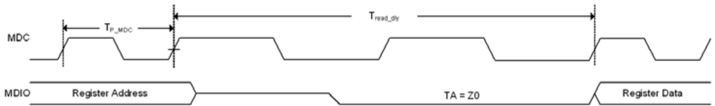
Figure 40: MDC Read Turnaround Delay
