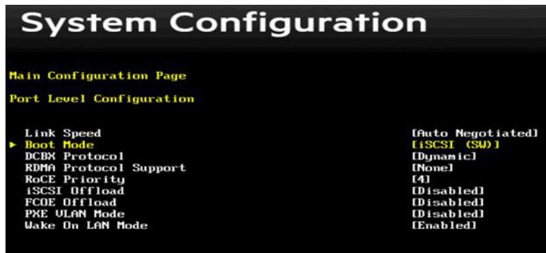
3. Return to the Main Configuration Page. Navigate to **iSCSI Boot Configuration Menu** → **iSCSI General Configuration**.
