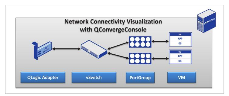
Figure 5. QConvergeConsole Plug-in Network Connectivity Maps
