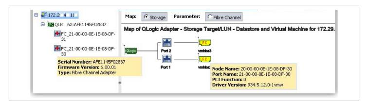
Figure 4. QConvergeConsole Plug-in Mouse Overs Provide Key Information
