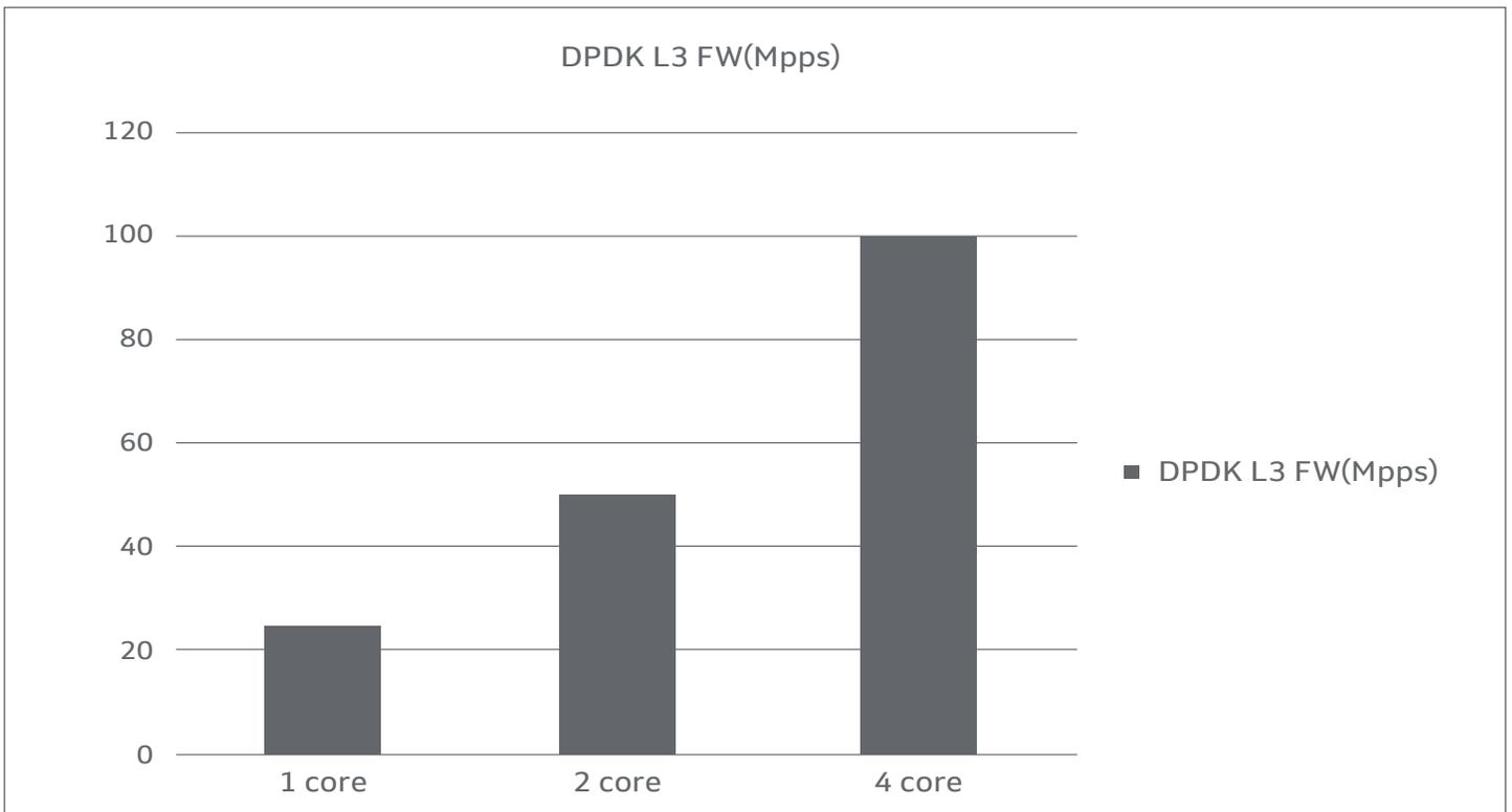
**Figure 3: OCTEON TX2 DPDK L3FW Multi-Core Scaling**
