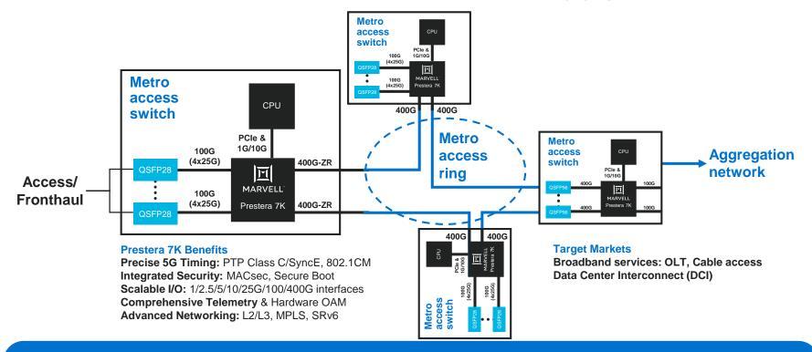
Ethernet switching in metro networks powered by 400G coherent pluggable optics
